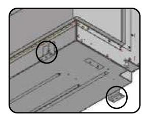
Determine the finished height and position that you want the appliance to be located. Build your base support taking into consideration the **50mm ventilation gap under the** appliance required on e810DS and e1030DS models (There is no ventilation gap required for the Octane DS models). Then place the appliance onto your constructed base and check that it is well supported.
