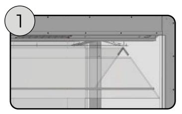
Start by applying the glass sucker to the centre of the effect glass. Begin lifting the glass up towards the triangular glass clip to slot in place.
