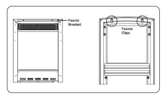
The cast frame can now be screwed to the appliance using the 2x screws supplied. The screw holes are located at the lower part of the frame. Once these are fitted, the fret panel can be fitted in front of this.
