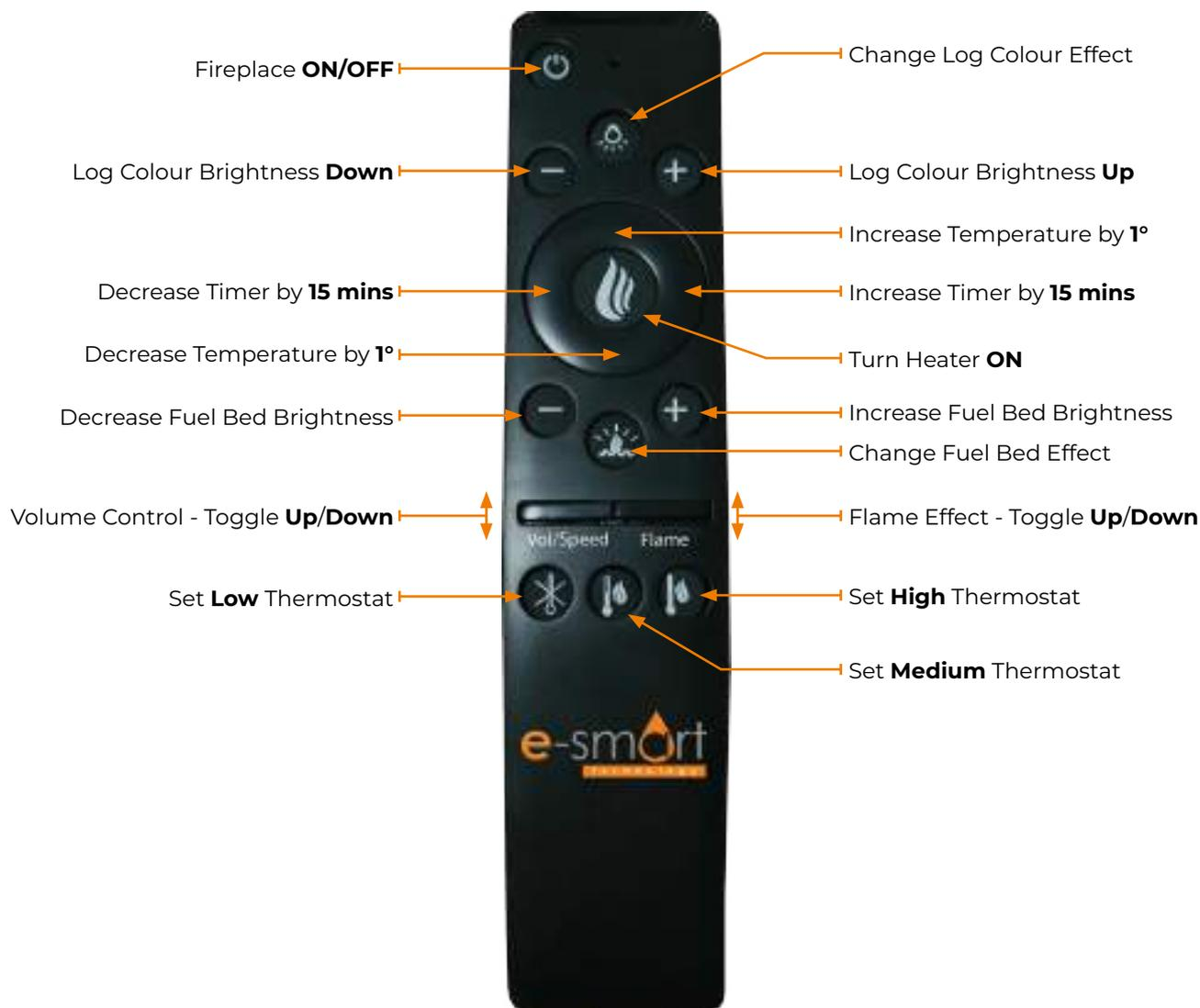
**2. Factory Reset:** To reset, press and hold the 'Change Log Colour' button until you hear a beep, then press and hold the 'Change Fuel Bed Effect' button until it beeps again. The reset process is complete.
