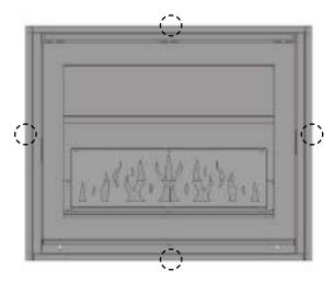
Above you will see suggested positioning for the magnets, although they can be positioned anywhere along the plaster kit to provide extra support.
