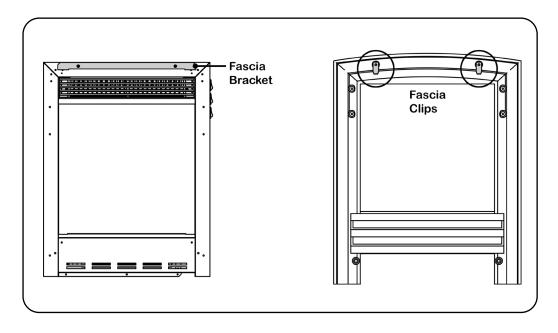
The cast frame can now be screwed to the appliance using the 2x screws supplied. The screw holes are located at the lower part of the frame. Once these are fitted, the fret panel can be fitted in front of this.
