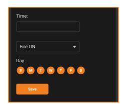
Input your desired time in the Time box, select the action (Fire On/Off/, Heater On/Off) you want. Deselect the day/s you don't want it to apply to, and press the Save button.
