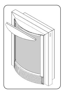
With the top plate now removed, slide the glass upwards to remove.
