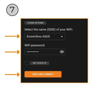
Select your router from the drop down box, and enter your router's password. Press the eye icon to double check for mistakes. Press 'Save and Connect'. Only select Static IP if advised by an IT professional.
