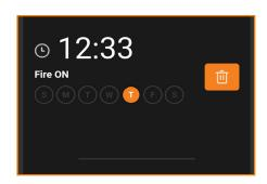
The above screen will now show your set timer. To delete the timer press the bin icon. To add an additional timer scroll down and repeat the process. Press the Back button to return to the Home Page.
