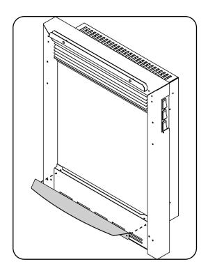
Our Strellar model comes with an infill plate and 2x screws, if you have an Oberon model you can skip to the section below and continue with the installation.
