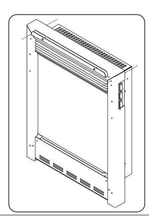
First attach the electrical lead to the power inlet on the back lower right, and plug into the mains power. Using the Cast Frame fixing kit, drill and fit the x 2 wall plugs and x 2 screw eyes to the inside of the wall opening.
