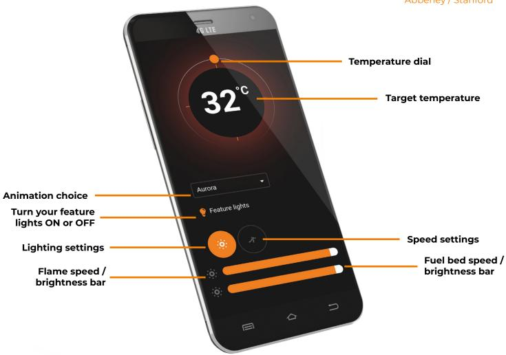
To adjust the desired temperature of your fire ensure that the heater is selected on the Home Page in the previous step. Then press, hold, and rotate the temperature dial to set the temperature.
