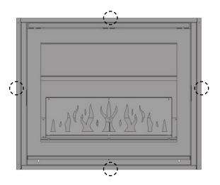
Above you will see suggested positioning for the magnets, although they can be positioned anywhere along the plaster kit to provide extra support.
