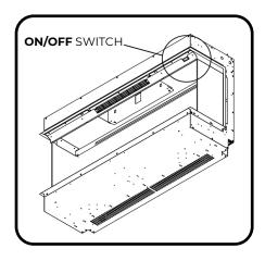
Make sure that your fire is plugged in and the switch is on. Then turn on your fire by pressing the ON/OFF switch to the 'ON' position.
