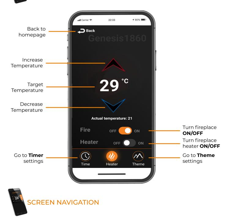
The Heater overview screen allows you to access all the key features of your fireplace. From this page you can turn your heater and fireplace **ON/OFF** and control temperature settings.
