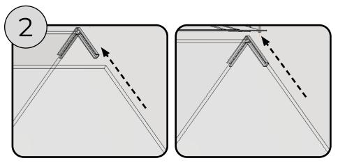
Line up the glass with the glass clip, and carefully push into place. The glass clips can be loosened on both sides to allow easier fitting.
