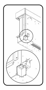
Determine the finished height and position that you want the appliance to be located. Then secure the wall bracket to the wall in the position you need using the wall plugs and screws provided. If you're not securing the appliance to a masonry wall you will need to use the appropriate fixings.
