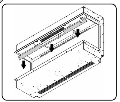
Slide out the side glass piece(s). Depending on the model, you may have to angle the side glass
