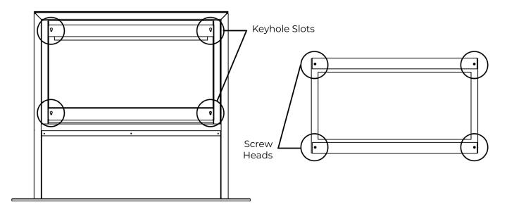
Now line up the screws and screw holes and slot them into each other, then allow the glass to drop into place.
