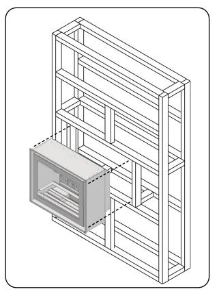
Once you have slid the appliance into place, you can then go about securing it in position by screwing it into the studwork frame. There are 4 holes located in each corner .
