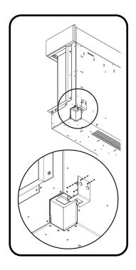
Determine the finished height and position that you want the appliance to be located. Then secure the wall bracket to the wall in the position you need using the wall plugs and screws provided. If you're not securing the appliance to a masonry wall you will need to use the appropriate fixings.
