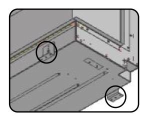
Determine the finished height and position that you want the appliance to be located. Build your base support taking into consideration the **50mm ventilation gap under the** appliance required on e810DS and e1030DS models (There is no ventilation gap required for the Octane DS model). Then place the appliance onto your constructed base and check that it is well supported.
