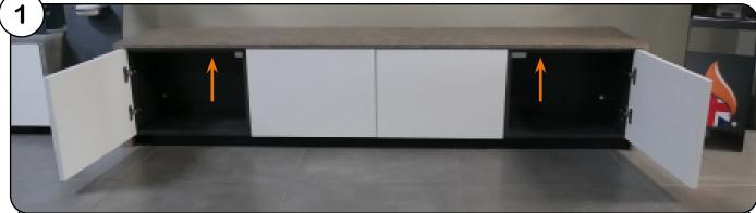
Place the top hearth accurately in place. Using the counter-sunk holes, screw into place. When screwing the hearth into place, ensure you do not push too firmly as this could result in the screws breaching the hearth.
